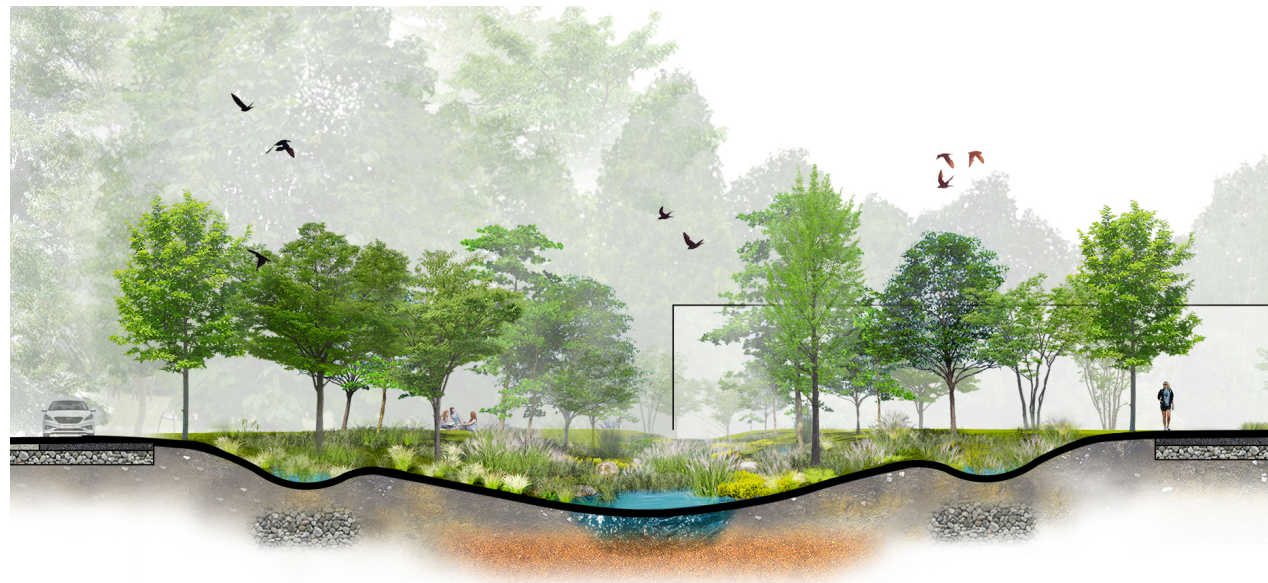
Figure 5-2 Cross Section Rendering of a Biofiltration Area With Wet Pool
